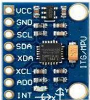
Fig. 3. MPU6050 - Gyroscope and Accelerometer
