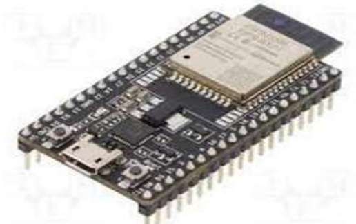
Fig. 2. ESP 32 - Microcontroller and Wifi
